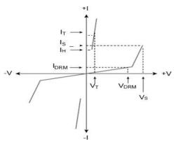
Stand-off Voltage -- Maximum voltage that can be applied to the TSS without operation **VDRM**
