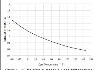
Figure 1. DC holding current Vs. Case temperature
