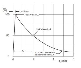
Figure 2. Pulse waveform
