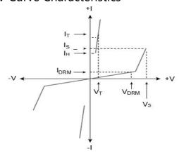
$V_{DRM}$ Stand-off Voltage -- Maximum voltage that can be applied to the TSS without operation
